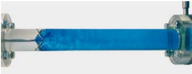
5% blue additive is dosed upstream of an Aquamix ( Re = 18000 )
