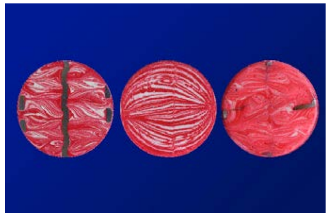
Cut views of epoxy resin mixtures produced under comparable conditions. The section on the left is of a CSE-X/8 mixture after L/D = 3 . The middle section was obtained using a helical mixer after six mixing elements ( L/D = 9.6 ). The section on the right shows a CSE-XC/4 mixture after L/D = 4 .
